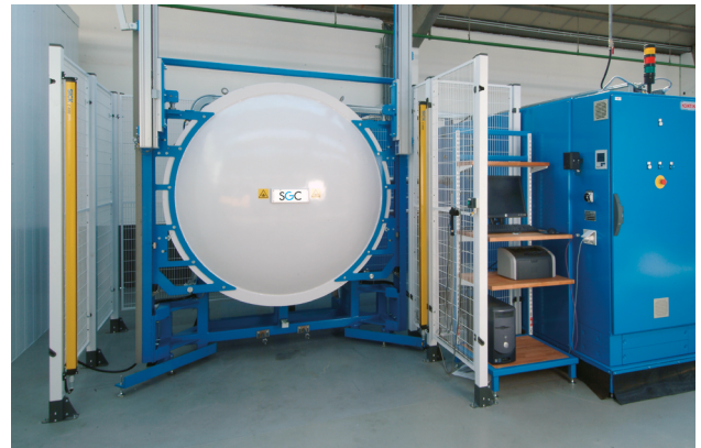
SF 6 filling and sealing station
